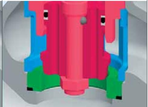
**Pressure-balanced valve plug**
