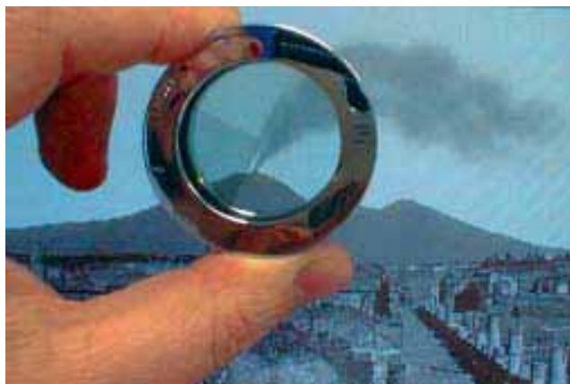
Fig. 4 Assessing a flue-gas plume with a Ringelmann scale
