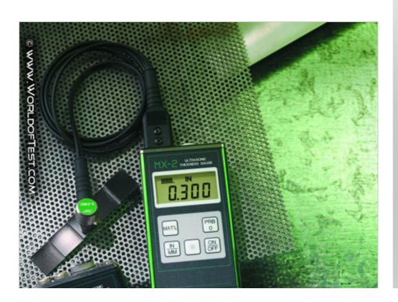
program allows the user to program the MX-2 for two additional set material types. Note: The material velocity must be known prior to programming.
