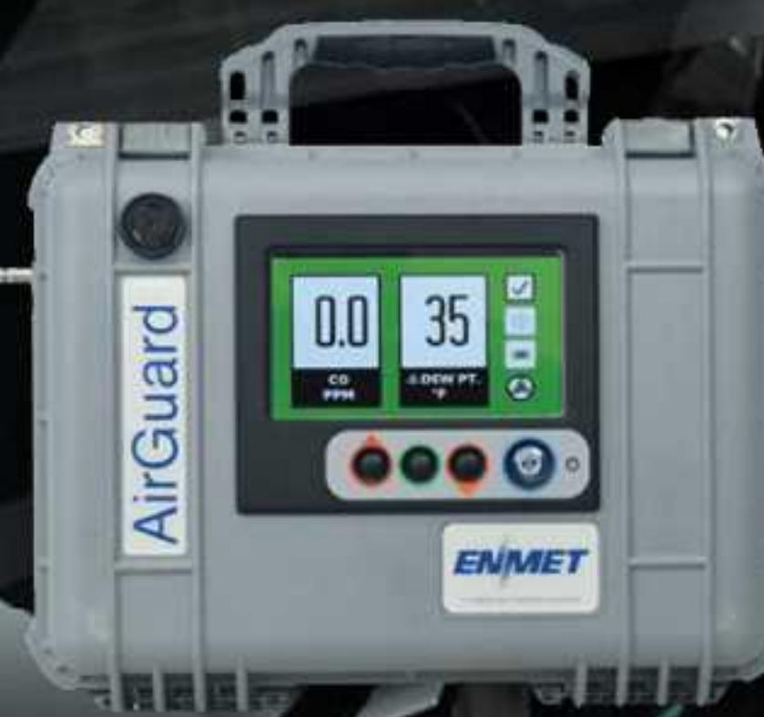
Portable Breathing Air Systems Portable Gas Verifier
