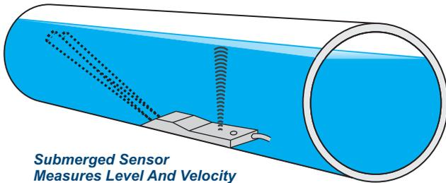
The MantaRay Portable Area-Velocity Flow Meter measures both Level and Velocity to calculate flow in an open channel or pipe. Calibration is simple: enter the pipe diameter or channel dimensions and the MantaRay automatically computes and displays the flow rate and total on its backlit LCD display.
