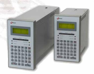
THE OMNI 3000 AND OMNI 6000 FLOW COMPUTERS ARE RELIABLE, EASY TO USE, AND UNIQUELY VERSATILE FLOW MEASUREMENT INSTRUMENTS. THEY ARE USER- CONFIGURABLE FOR SINGLE OR MULTI-RUN OIL AND GAS APPLICATIONS. TYPICAL PRODUCTS MEASURED INCLUDE: CRUDE OILS, REFINED PRODUCTS, NGLS, LPGS, ETHYLENE, PROPYLENE, NATURAL GAS, AND SPECIALTY GASES, SUCH AS O2, N2, H2, H2O, AND CO2.
