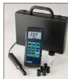
Complete with 0.8" (20mm) probe on 13ft (4m) cable, membranes, protective holster with stand, 9V battery, and carrying case
