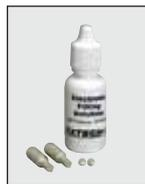
PH113 Reference Refilling Solution Kit for PH115 Refillable pH electrode module
