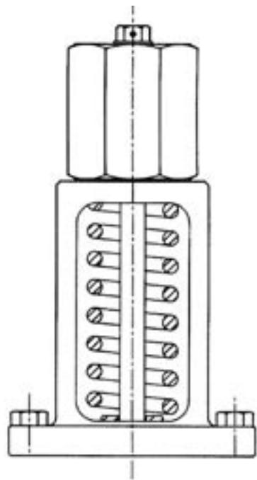
**Vite di blocco • Test gag**
