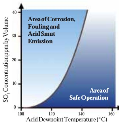
The relationship between the Rate of Acid Build-up and Flue Gas Temperature
