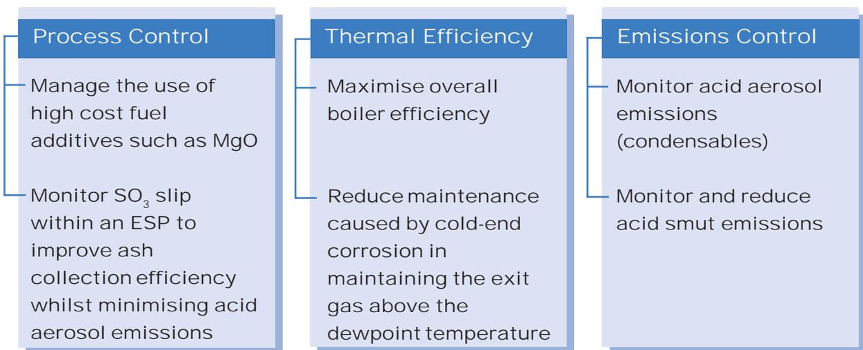
**When compromising combustion efficiency is not an option, the Acid Dewpoint Temperature becomes a vital measurement and process control parameter.**
