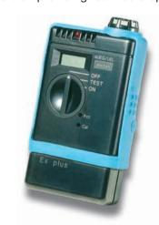
tion time, or the long-time monitoring version providing up to fifteen hours operation time. The explosion proof rechargeable battery packs can easily be changed in seconds, no tools needed. This allows users to convert the minidetector into a long-time monitor even in hazardous areas. Tracer Tracer
