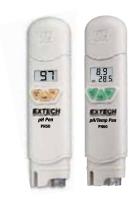
Model PH50 Measures pH Model PH60 Measures pH and Temperature
