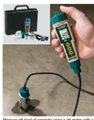
Measure pH level of concrete using a pH meter with a flat surface pH electrode plus a metal weight probe guard for stability and protection
