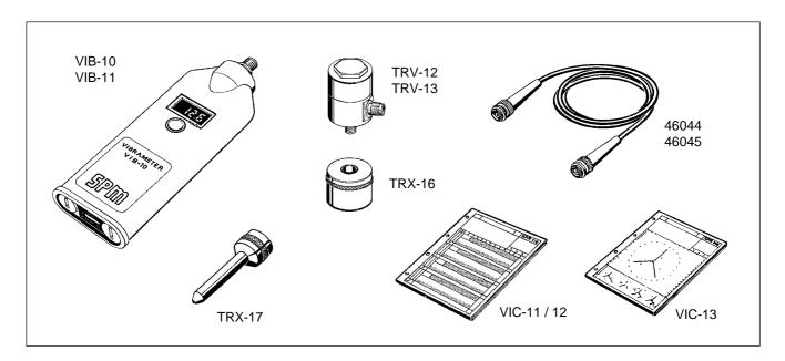
Vibrameter VIB-10 (VIB-11) has been designed as a simple diagnostic tool for preventive maintenance. The instrument and the monitoring technique are based on the recommendations of ISO and the equivalent national standard organizations BS, VDI, etc.
