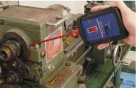
Use the contact probe to listen to bearings, gearboxes, valves, steam traps etc. Easily compare noise levels between like objects.
