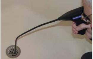
Inspect drains for blockages and lost items. Inspect behind walls for water or insect damage. Watertight tips eliminate worry of damage.
