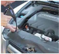
Inspect pistons, cylinder walls and T-belts. Look inside A/C ducts for mold and mildew buildup. Find oil and water leaks in hidden areas.
