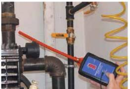
Using the air probe you can locate pin-hole leaks up to 10 feet away. Find pressurized or vacuum leaks on all types of gases such as air, freon, nitrogen, propane, etc.
