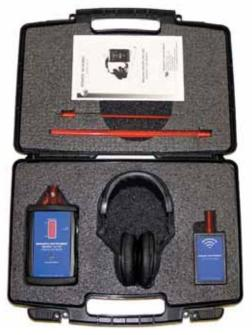
UltraPro AG500 System includes: Detector, Headset, Air and Contact Probes, Tone Generator, Batteries and Latching Carrying Case.
