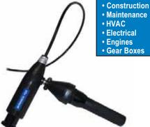
Monarch FSX Series Flexible Fiberscopes require an optional external light source. (Order the Scorpion Xenon flashlight). Only 6mm diameters are available in lengths of 24, 36, 48 and 60 inches.
