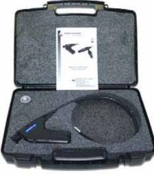
Monarch FSI and FSX flexible fiberscopes include padded latching carry case with operation manual (optional clip on mirror shown).
