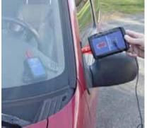
Place the tone generator inside a vehicle, closed vessel, container or building and search for leaking seals and gaskets around doors and windows.
