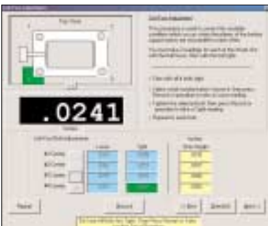
Soft-foot routine eliminates time-consuming alignment problems caused by soft foot.
