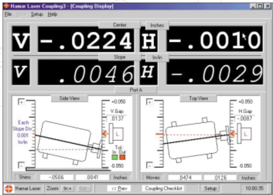
Final alignment screen shows alignment status, shim calculations and horizontal moves needed for proper alignment.
