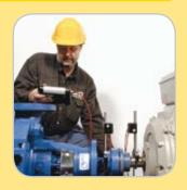
display through the entire measurement procedure. Even though the technology inside is rather advanced, the measurement principle is straightforward. It is based on the "reverse indicator method" with two laser/measuring units mounted on each side of the coupling.
