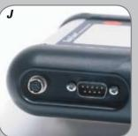
Countersunk connectors, well protected against external damage.
