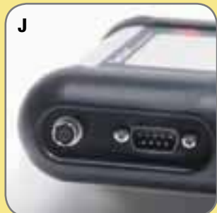
Countersunk connectors, well protected against external damage.
