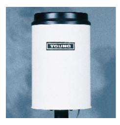
Catchment area of 200 cm<sup>2</sup> and measurement resolution of 0.1 mm meet the recommendations of the WMO. Extensive use of molded thermo-
