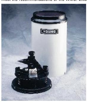
plastic components ensures maximum performance and value. Leveling screws and bullseye level are built-in for easy and precise adjustment in the field. Measured precipitation is discharged through a collection tube for verification of total rainfall. Model 52202 is heated for operation in cold temperatures. An unheated version, 52203, is available for use in moderate climates.
