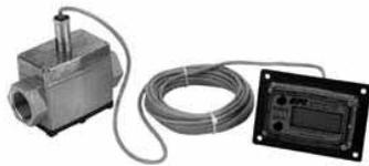
The Standard Remote Kit Assembly modifies GPI Electronic Digital Meters for applications in specialized situations including remote indication and high or low fluid temperature metering applications. This kit also provides the versatility of panel mounting of the LCD readout up to 300 ft. from the turbine housing and sensor.
