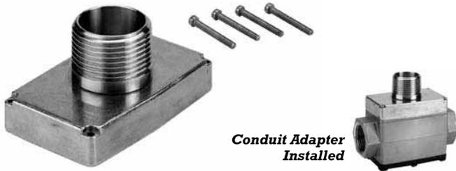
The Conduit Adapter allows you to enclose wiring from the magnetic pickup. The kit includes a turbine meter cover with a 1 inch male NPT conduit fitting and screws for plastic or metal installation.
