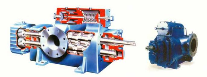
Bulk liquid transfer pumps utilising two contra rotating screws providing a smooth pulse free flow. Each screw is accurately located between bearings providing a physical gap between each screw and between the screwset and casing, this providing a positive displacement pump which does not require internal lubrication from the pumped liquid.
