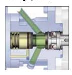
□ DIN 24960, materials and version as requested, fluids with a tendency to harden / reaction when in contact with surrounding air, inlet pressure = 6 bar; T<sub>max</sub> = 150 °C.
