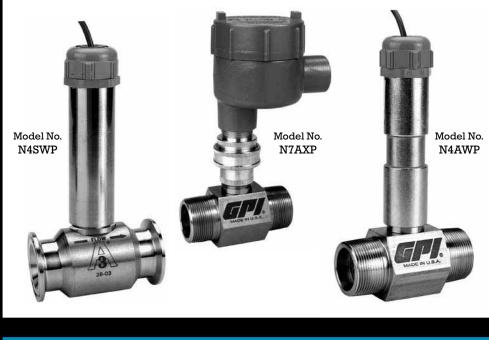
Pickup Enclosures are optional on G Series Meters. Choose from four pickup enclosures. Models N4A and N4S are weatherproof enclosures. For explosion-proof enclosures, choose N7A for the enclosure without terminal strip or the N7AT with terminal strip.
